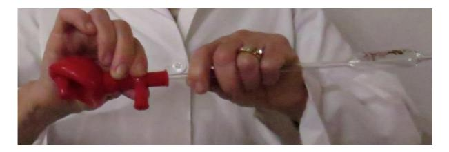
When drawing liquid up into the pipette, always ensure that the tip is well below the liquid surface, in order to avoid sucking air and possibly contaminating the filler.
